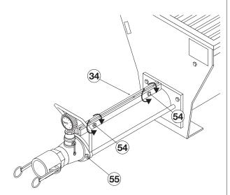
Remove the material delivery header, loosening the retaining nuts of the stay rods (55).
