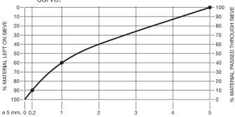
for example, use aggregates that have particle size: 1/3 between 0 and 1 mm inclusive 1/3 between 1 and 3 mm inclusive 1/3 between 3 and 5 mm inclusive.
