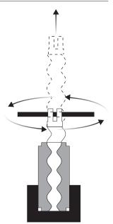
This check is carried out by resting the screw on a horizontal surface and checking that the distance of the impeller tips from the surface is not less than **(56)**:
