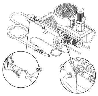
Then connect the spray gun to the end of the material hose; when using the gun for traditional mortars (code
