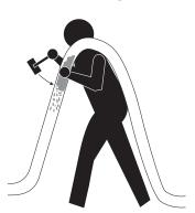
Start the pump for a few moments and ensure that the hose is free of the plug: the material should flow out freely.
