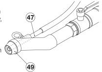
Disconnect the hoses from the mortar pump and insert a cleaning sponge into the end of the hose.
