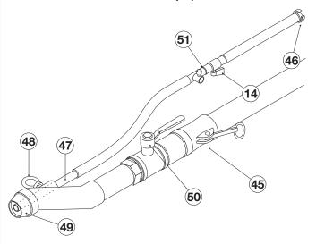
By way of general information, using nozzles and spray tips with a smaller diameter results in a wider spraying rose of the material and vice versa.
