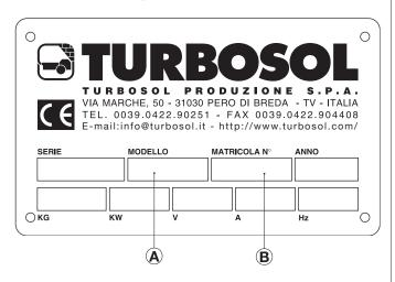
The type of machine (A), its serial number (B), and data on the machine's operating power are printed on the manufacturer's registration plate.
