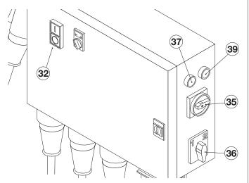
Start the mortar pump by pressing the start/stop button **I/O** (32).
